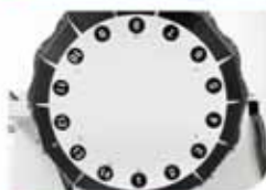
14 Tools Turret Type ATC ▶ Tool change is fast accomplished in only 1.8 seconds (tool to tool) and 2.8 seconds (chip to chip)
